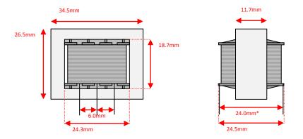
Please Note: Pins are wire spills fixed to the outside of the coil – actual distance between rows will vary with thickness of coil.
